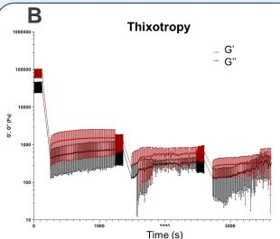
**B: P22 Thixotropy**: Partial but rapid viscosity recovery after shear stress, preventing collapse and ensuring 3D stability.
