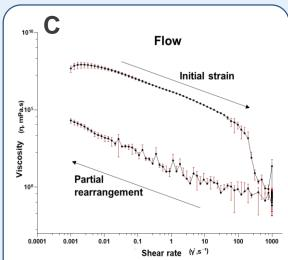
**C: P22 Flow curves:** Shearthinning profiles, essential for printability, extrusion fidelity, structural integrity
